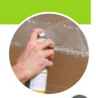
Alternatively, the ASK DS770 spray adhesive can be used. However, after the sheet has been attached to the no more corrections to the desired position.
